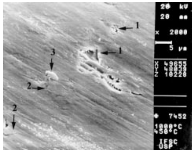
Fig. 5 Photomicrograph of alloy A1, by MEV, after two body abrasion tests. Heat treatment: sample T2 (Table 3)
